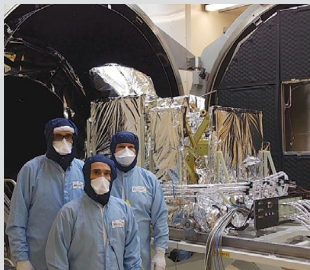
Sentinel-3B SLSTR FM2 at RAL ready to start thermal valance/vacuum testing at Rutherford Appleton Laboratory/STFC facilities (Selex ES)
