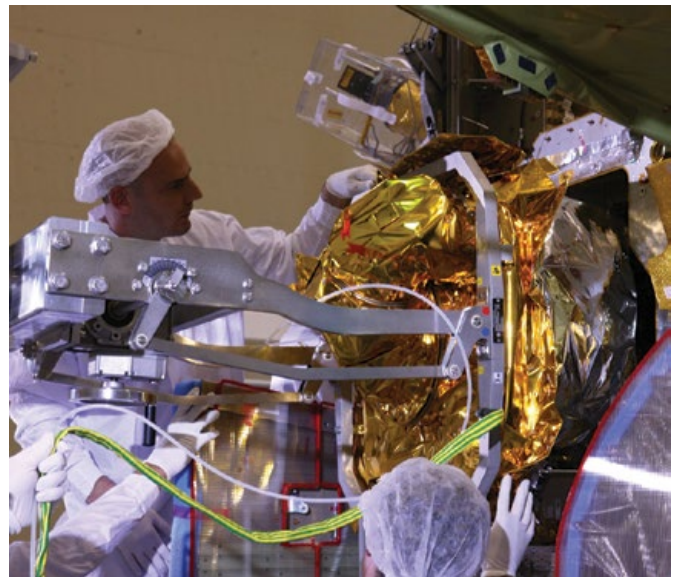
↑ The TESAT-Spacecom EDRS-A Laser Communication Terminal is integrated on the Eutelsat-9B satellite in Toulouse, France (Airbus Defence & Space)
