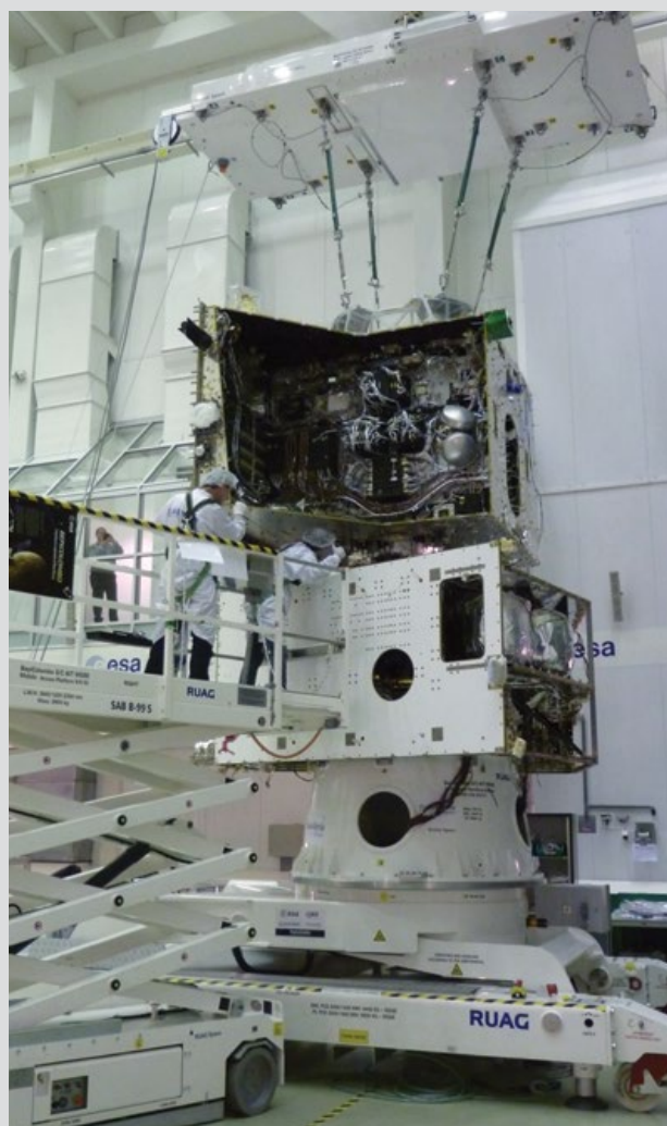
First mating of BepiColombo MPO/MTM Flight Models
