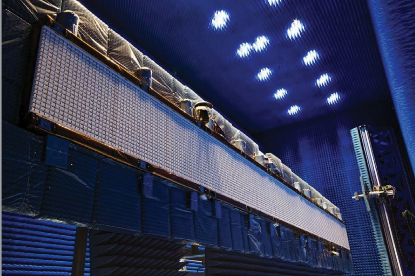
The Sentinel-1B antenna during characterisation tests (Airbus Defence & Space)
