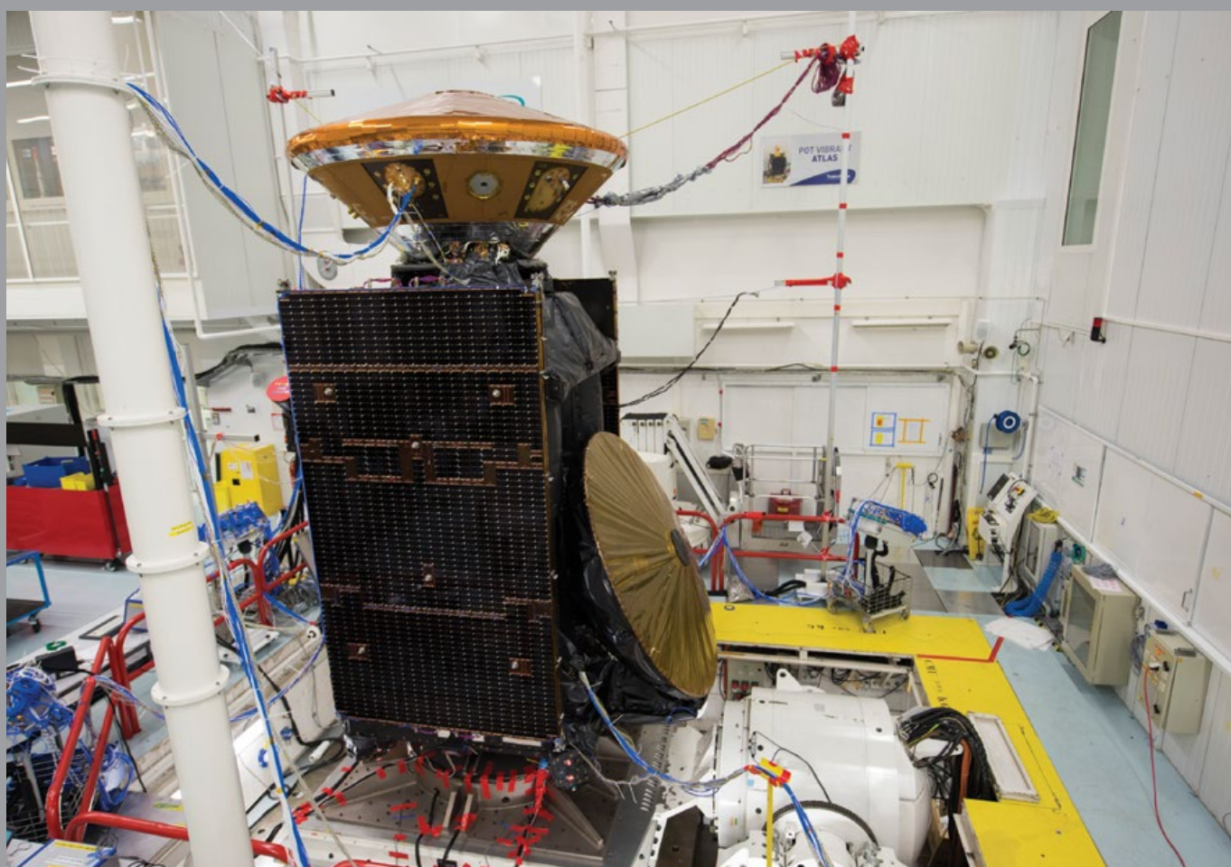
The ExoMars 2016 integrated Spacecraft Composite, consisting of the Schiaparelli entry vehicle atop the Trace Gas Orbiter, in preparation for sine vibration testing
