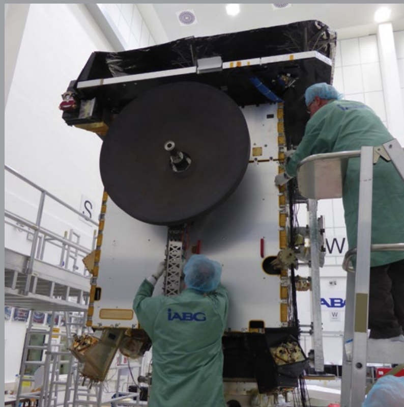
Solar Orbiter spacecraft Structural and Thermal Model at IABG test facilities
