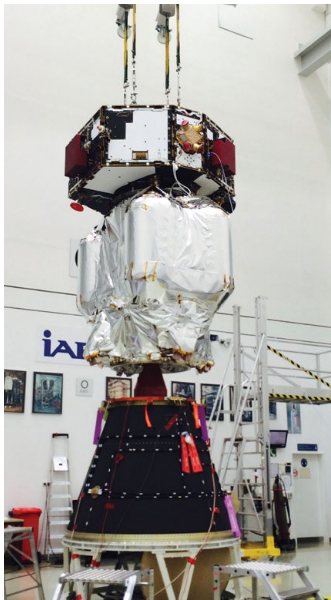
↑ The LISA Pathfinder science module and propulsion modules on the Vega launch vehicle adapter at IABG, Ottobrunn, in June (ESA/U. Ragnit)
