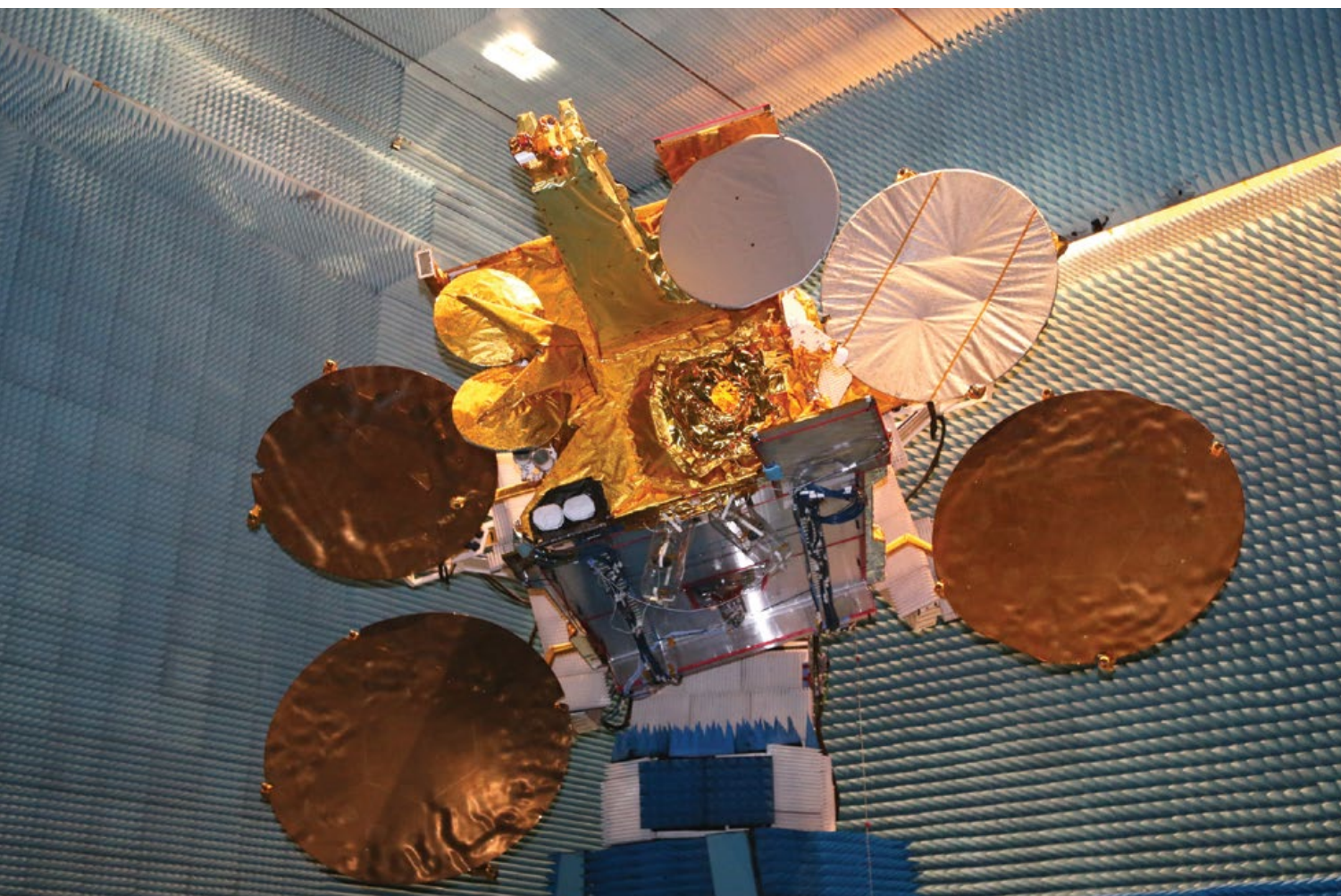
↑ The Eutelsat-9B satellite with its EDRS-A payload in the anechoic test chamber in Toulouse, France (Airbus Defence & Space)
